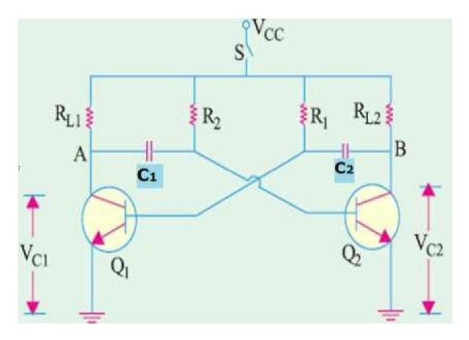
This astable circuit consists of two transistors, a cross coupled Feedback network, and two capacitors and four resistors.
